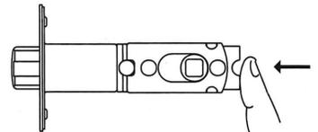
1D. To reset the latch to 2-3/8" backset, push spindle cam to the left edge of the adjusting hole.
