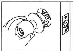
Before proceeding, make sure spindle hole in the latch is oriented correctly. For keyed sets, orient key cylinder as shown.
