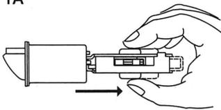
1A. If 2-3/4" backset is required, pull spindle cam all the way to the right edge of the adjusting hole.
