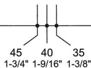
Mark 1" (25.4mm) hole at center of door edge.
