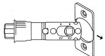
2C. With Drive-In Latch installations, rotate latch faceplate clockwise 20 degrees and pull plate off back of latch (no faceplate is needed).
