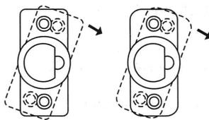
2B. For Radius Cornered Mortise Faceplate, remove squared mortise plate. Rotate the Square Cornered Latch Faceplate clockwise 20 degrees and pull faceplate off back of latch. Replace with Radius Cornered Mortise Plate.
