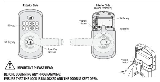
There are two ways to enter the programming mode. First, by pushing the Program Button (shown above in the diagram). A second method is by creating a Programming Code, which allows you to enter the programming mode if you don't have access to the interior of the lock. Please follow the instructions starting in Page 2 or follow the table reference below to begin programming.
