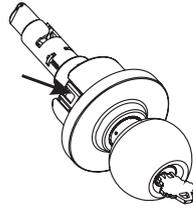
**A3:** Press slider with left thumb or other tool and keep press, then release your right hand from key.
