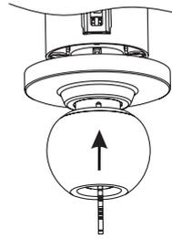
**C6:** Push knob into position and pull knob to make sure catch fully engages knob.
