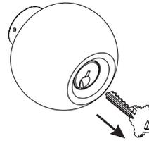
**C1:** After changing a new cylinder, pull out the key to confirm the key and keyway direction are correct.
