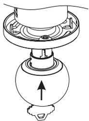
**C3:** Erect the lock, hold key and put knob onto spindle, you may need to shake the key slightly to lead knob gets in easily.
