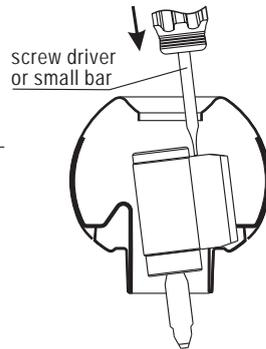
**B3:** Or you can knock the cylinder with a screw driver to push knob cap out as shown. It is easy to remove knob cap this way.
