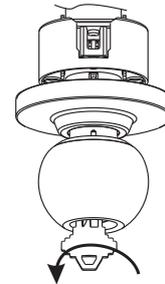
**C7:** Turn key back counter clockwise. Not that if you turn key in wrong direction, you can not pull key out. In this case, you need to remove the knob and reinstall it (see A1-A5 and redo these steps).
