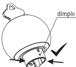
**B2:** Nip this side, force dimples open and pull knob cap. It is easy to remove knob cap this way.
